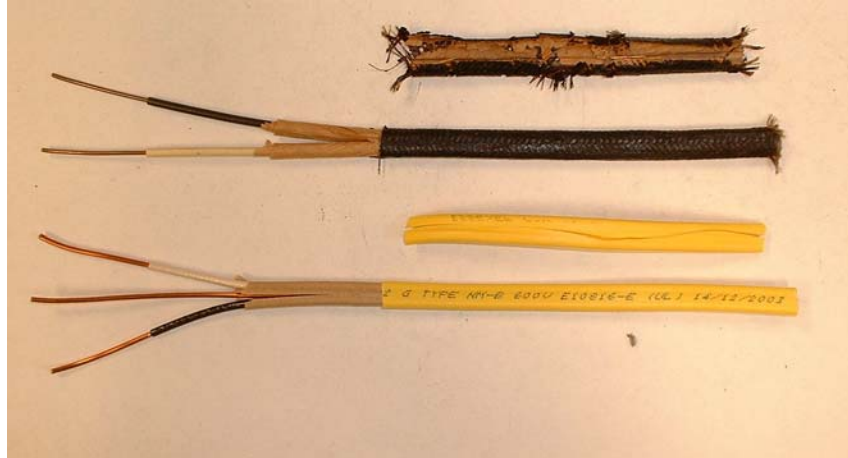
Fig. 4 – Older Cloth Braid and Newer NM-B Jacketed Cable
